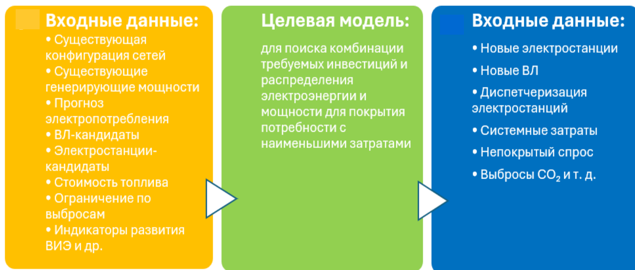
Diagram 142. Structural scheme of modeling scenarios for development of Kazakhstan's energy system until 2035
